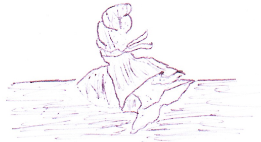
Step 4: Twist the bag and inner liner and fold in half (gooseneck) and tie again
