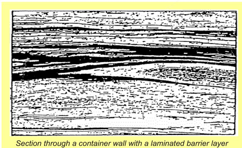
*Section through a container wall with a laminated barrier layer*
